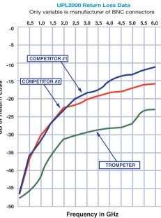
NOTE: Test setup includes one foot Belden 1505A coaxial cable with BNC plug each end plus adapter and terminatio
